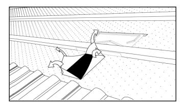
3. Lay the next course of tiles, overlapping the Versa-Tile on each side and compressing the foam filler. It may be necessary to remove adjacent tile nibs to prevent tiles "kicking-up". Fix adjacent tiles where necessary.
