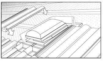
2. Fit the Versa-Tile in position and nail to the batten.
