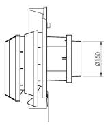
SUITABLE FOR ROOF PITCHES OF BETWEEN 20° AND 60° -FOR PITCHES ABOVE OR BELOW THIS CONSULT PASSIVENT TECHNICAL SERVICES
